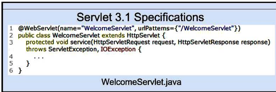
Diagram 7.9: Servlet 3.1 specifications where deployment descriptor is optional
