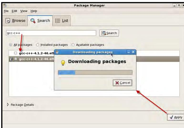
Diagram 9.1.8: Installing gcc-c++ package
